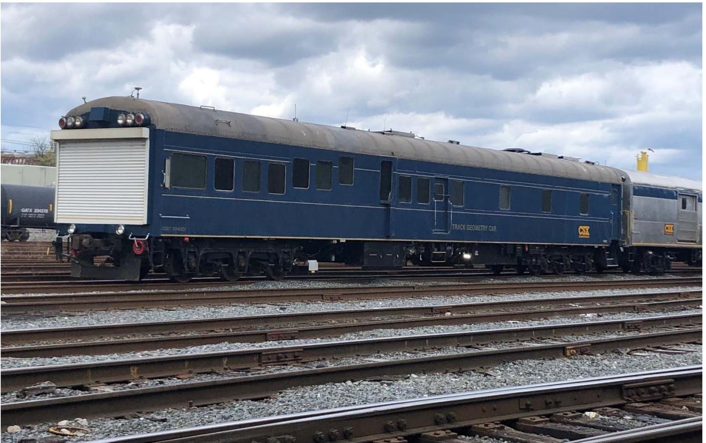
Seen on April 16, 2021 at Locust Point in Baltimore was **CSXT 994302**, a Track Geometry Car originally built by ACF in 1942 as C&O passenger car 817.
